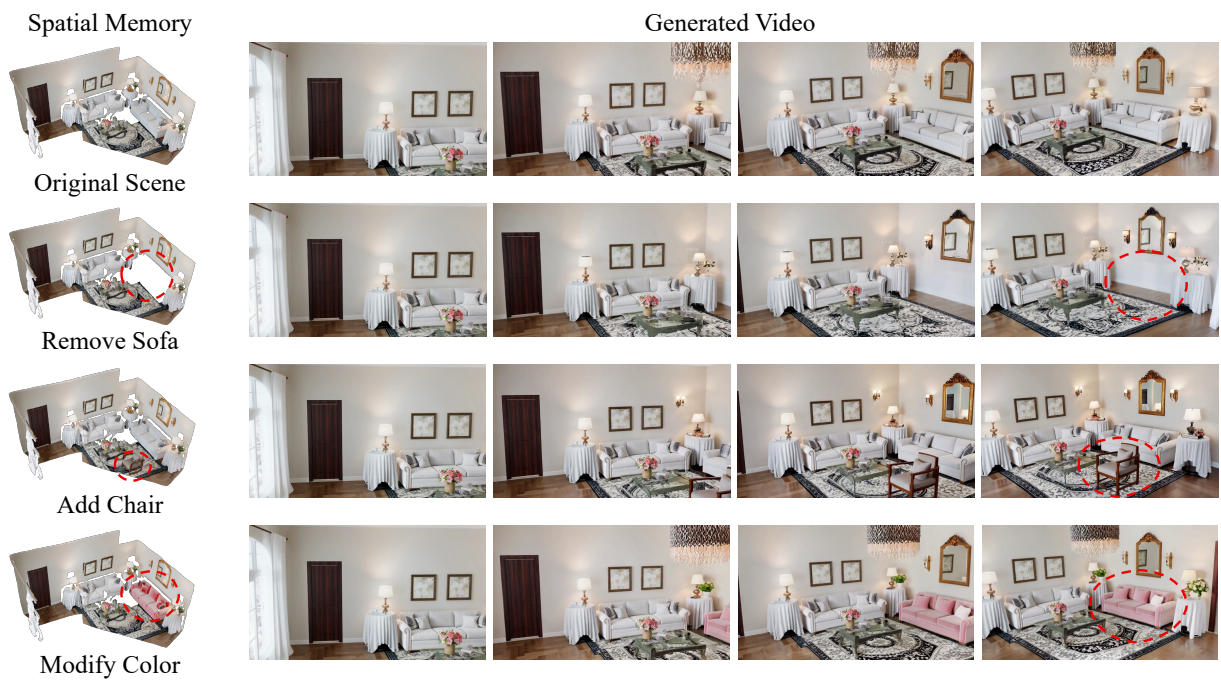
Figure 8. Demonstration of 3D-aware interactive editing. By directly modifying the spatial memory (i.e., the scene point cloud), users can achieve geometrically precise edits in the generated videos, such as removing an object (2nd row), adding a new object (3rd row), or altering object attributes (4th row).
